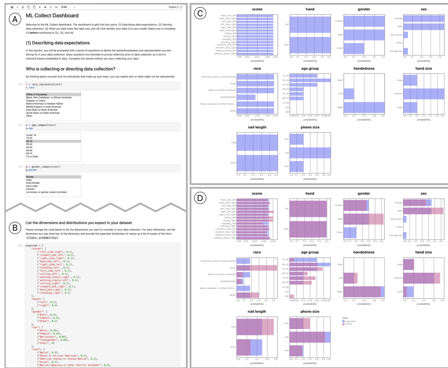
Figure 2. (A) Dashboard prompts practitioners through designing their datasets. (B) Before collection, the dashboard prompts documentation of expected distribution. (C) These are visualized as histograms. (D) As data is collected, true distributions (pink) overlay expected distributions (blue), highlighting divergent patterns.
